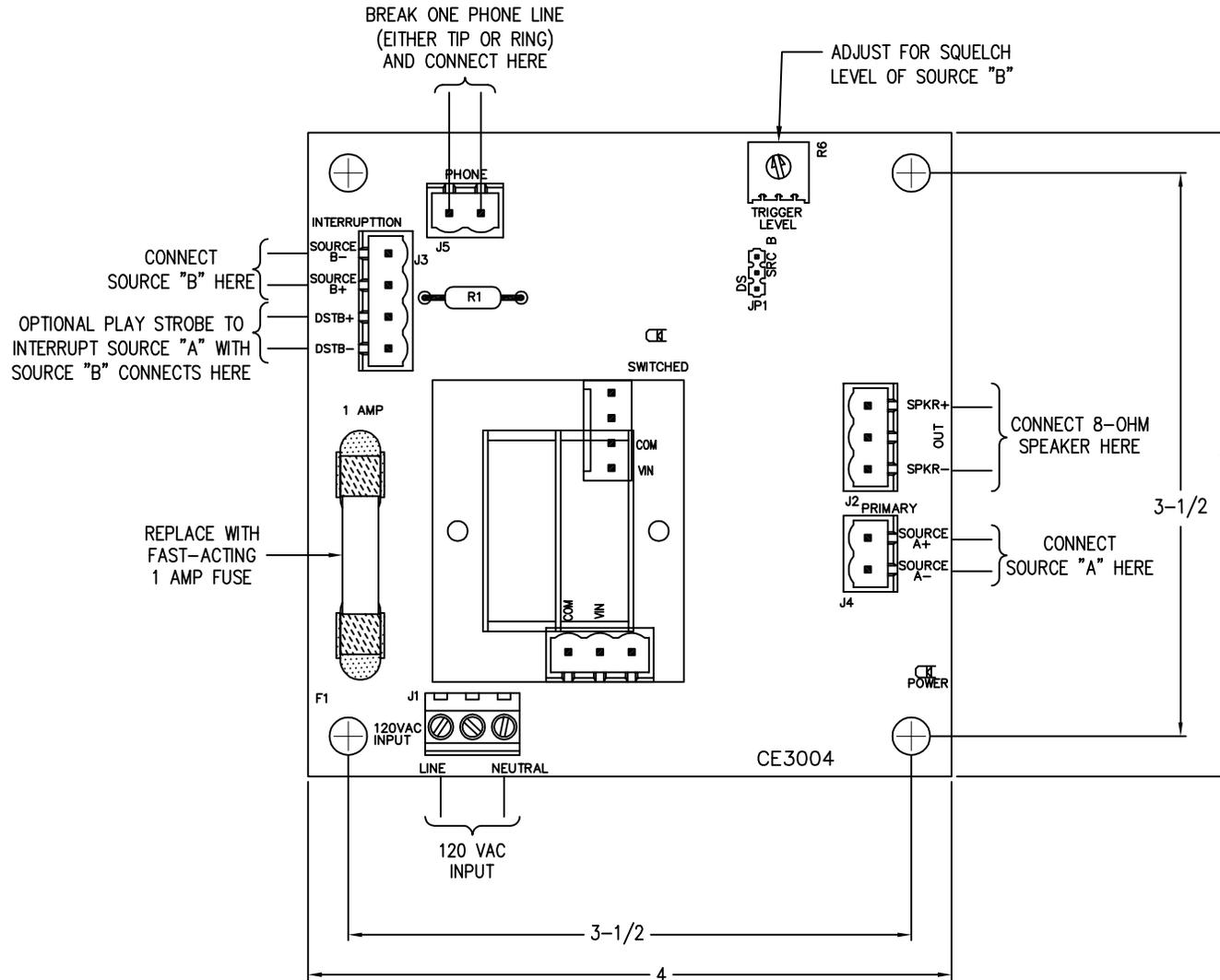
The speaker switch board allows for the use of and I/O source to be switched. The continuous audio source "A" is interrupted by the "B" audio source. Typical uses are with voice annunciator, intercom, and elevator music.
