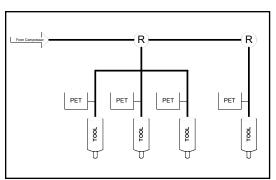
tool. The regulator is labeled "R" in this diagram. The pressure fitting on the PET will accept 1/4" O.D. diameter tubing.
