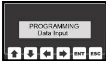
This unit is capable of receiving 40 input bytes. The user can select which groups of information are actually received.
