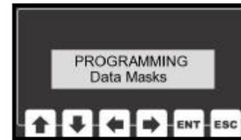
A few different automatically selectable data masks are resident in memory. By selecting one of these default masks, the user can set the input and output data to one of several different defaults.
