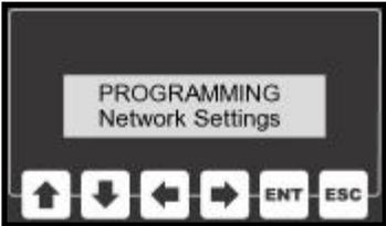
The menu system is broken down into a few different sub-menus. Select "Network Settings" from the main menu and press the ENT key.
