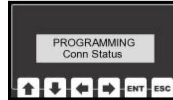
The module status and network status can be displayed by this unit as a means of trouble shooting this device.
