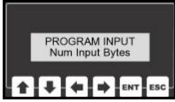
To set the number of input bytes, the user will want to select Num Input Bytes from the Data Input sub-menu. After pressing the ENT key, the user can use the arrow keys to set the number of input bytes. Pressing ENT will save this value. ESC will allow the user to exit without saving a new value.
