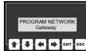
The Gateway setting holds the address of the device that will allow this unit to send and receive messages with devices that are not on the local network.
