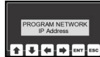
The current IP address will be displayed at this point. In order to change the address use the LEFT and RIGHT arrow keys to select any given digit in the address and then use the UP and DOWN
