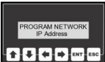
This step can be skipped if IP addresses are assigned dynamically by the network. If the connection type is static, select "IP Address" from the sub-menu and press the ENT key. Using the arrow keys, edit the IP address for the unit. Please consult the IT director for this value.
