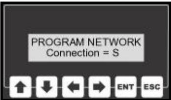
The the "Network Settings" sub-menu select "Connection" and press the ENT key. The connection type can be set to either static or dynamic. If dynamic is chose, the network should automatically select an IP address. If static is chose, an IP address will need to be programmed into the unit.
