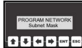
Next, from the networking sub-menu, select "Subnet Mask". The Subnet Mask helps the unit determine which IP addresses are local and which lie beyond a Gateway.
