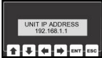
In the main operating mode, the display will show the unit's IP address.
