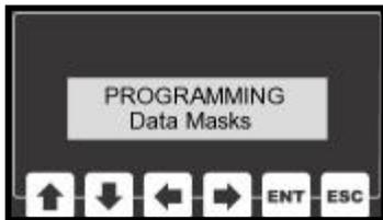
The data input and data output menus allow user to select which data bytes to send/receive and also where those bytes will be located in the input and output strings.
