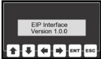
An additional human-machine interface (HMI) is added to AQ Wireless systems that are network enabled. The human-machine interface consists of an 2-line by 16 character backlit LCD display and a six-button keypad. During power-up, the display on the HMI will display the firmware version contained inside the microprocessor's memory.
