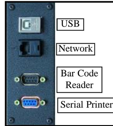
This network card comes with additional connectivity that standard AQ Wireless units do not have. The USB connector is available on standard AQ Wireless units. Please consult the AQ Wireless manual for more information about that functionality of that connector.
