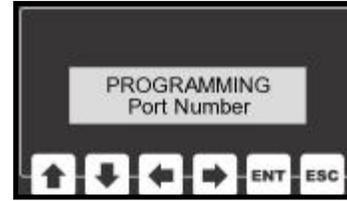
The Port Number sets the service port value that is used to connect to the ACOP system.
