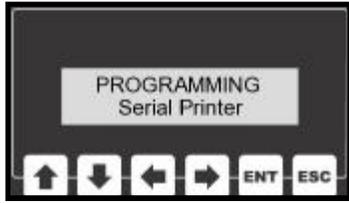
A serial printer can be connected to the 9 pin DSUB connector on the side of this unit. In the programming menu, a user can turn on this printing function by selecting Serial Printer from the programming menu.
