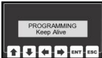
This unit expects to see messages from the client on a regular interval. The Keep Alive value defines the amount of time that this unit will wait to see a message before closing the socket.
