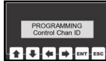
After pressing the ENT key, the alpha numeric field will appear on the display. The Up and Down arrows will allow the user to change each individual character. The Left and Right arrows will allow the user to select a new character to edit.
