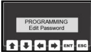
In order to gain access to the programming menu, the user must enter a password. The password is a four digit (numeric) code.
