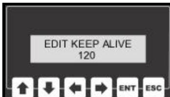
If a data message does not need to be sent within this time interval, the client should send a keep-alive message.
