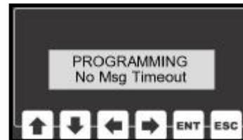
In a system where a keep alive messages are not desired, the No Message Timeout can be implemented to close the socket if communications are lost.
