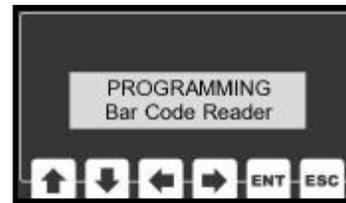
A bar code reader can be used to program items on the fly as the assembly process changes. In order to use a bar code reader with this system, the bar coding function must be turned on through the programming menu.
