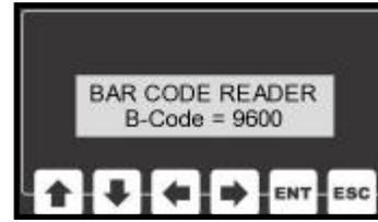
After Bar Code Reader has been selected from the program menu by pressing the ENT key, a baud rate can be selected by using the arrow keys. If a bar code reader is not being used, this function can also be turned off.
