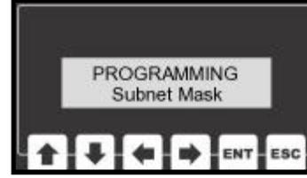
The Subnet Mask is used to identify which part of the IP address is the network ID and which part is the host ID. This is accomplished by a logical bit-wise ANDing of the IP address and the netmask.
