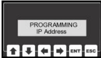
It's important that each device on the network has it's own unique IP address. In order to edit this interface's IP address, select Programming IP Address from the main menu and press enter.
