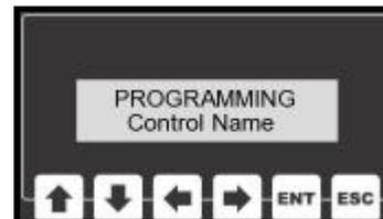
The ESC key can be pressed any time during the editing process allowing the user to return to the main menu without
