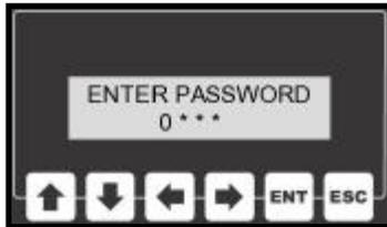
Use the network user interface and enter the program mode by pressing the ENT key. The unit will prompt the user for a password at this point, the default is "0 1 0 4". Using the keypad, enter the password
