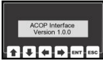
When the ACOP network interface powers up, the display briefly shows the firmware version information and then the unit enters its operating mode.
