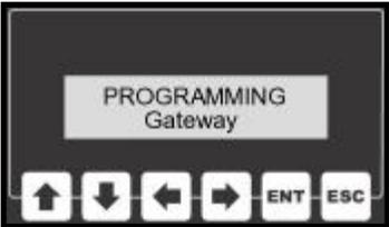
The Gateway setting holds the address of the device that will allow this unit to send and receive messages with devices that are not on the local network.
