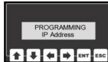
While entering the password, the left and right arrow keys will move the cursor back and forth. The up and down arrows will raise and lower the value of the digit that the cursor is highlighting.
