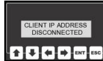
Press the ESC key to return to the main screen. Using the UP/DOWN keys the user can choose to view either the unit's IP address or the client's.
