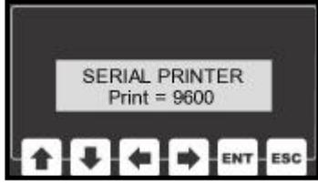
Inside the Serial Printer menu, a baud rate can be selected for communications with the serial printer or this function can be turned off entirely. This setting can be altered by using the arrow keys.
