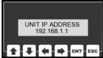
In the main operating mode, the display will show the unit's IP address or the client's IP address. Using the UP or DOWN keys the user can select which IP address is visible.
