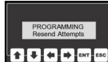
When a message is sent to the ACOP system and an acknowledgment is not received, this unit will wait for an amount of time defined by the ACK
