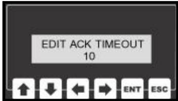
The Message Timeout setting sets the amount of time that this unit will wait for an acknowledgement before re-sending the message or closing down the socket.
