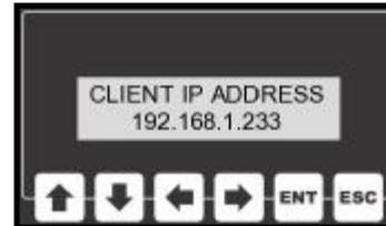
If a connection is active, this screen will display the IP address of the client's computer.
