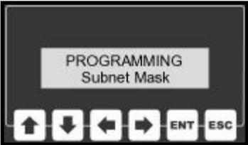
The Subnet Mask helps the unit determine which IP addresses are local and which lie beyond a Gateway.
