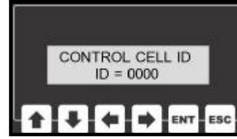
To change one of these alpha-numeric values, select the appropriate control field from the programming menu and press the ENT key.
