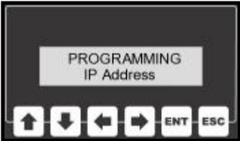
Scroll through the program menu until the unit displays IP Address. Press the ENT key to view the unit's IP address. Using the arrow keys alter this address to the desired value (please consult your IT group for this address). Press the ENT key to store the value.
