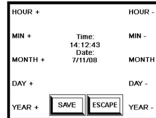
If the EDIT key was pressed, a screen will appear that shows the time and date but also has assigned several editing features to the soft keys to the left and right of the display. The soft keys on the left side of the display will all add one to the hour, minute, month, day or year depending on the key that is selected. On the right side of the display, the keys will all subtract one from those same values.
