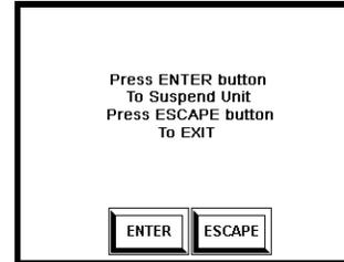
While the unit is suspended, it will ignore cycles, batches and rejects.
