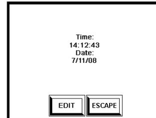
A screen will appear that shows the current time and date. If these values need to be edited, the EDIT button can be pressed. The ESCAPE key can also be pressed to exit this routine.
