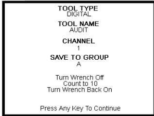
*Turn off the wrench for 10 seconds, then turn in back on.*
