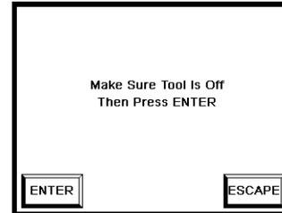
Then you'll be prompted to run a fastener and press enter. At this point, run the tool on a typical fastener and press enter. The transducer will automatically create a parameter set (group) that will work with the previous fastening.
