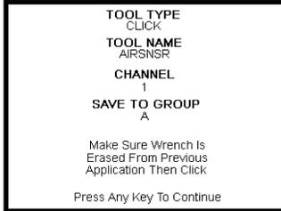
For wireless transducers (air tools), the user will be prompted to hold the learn button on the transducer until it enters the learn mode. The Rx/Tx LED on the transducer will toggle to signify that it has entered into the learn mode. When the button is released, the display on the AQ wireless will give the user feedback on the progress of the learn process.
