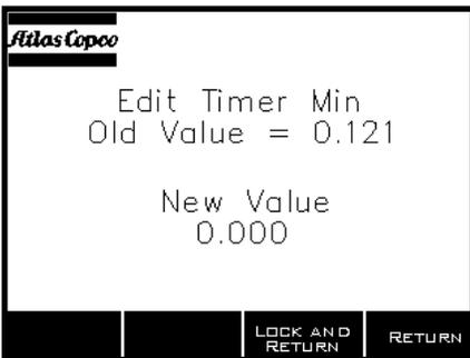
After an item from the parameter list is selected, another screen will appear showing that item's original value. On the screen will also be a new value. A user can edit the new value by typing the desired value on the keypad.
