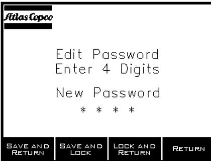
Once the new password is entered, the value can be saved by pressing either the SAVE AND RETURN soft-key or the SAVE AND LOCK soft-key. (The SAVE AND LOCK soft-key will lock the unit and place the screen back into the MAIN mode).
