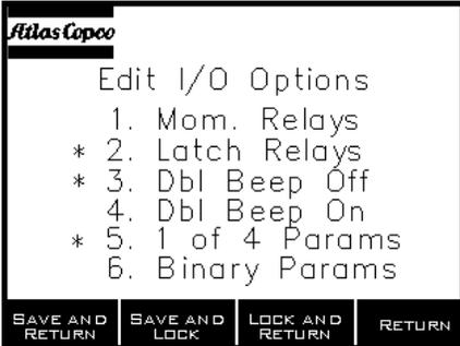
Numbers 1 and 2 both relate to how the relays work. If 1 is selected, the relays will be momentary and will come on for 200 milli-seconds each time they are activated by a change in status. If the relays are set to latching (2) the relay will remain on until the beginning of the next cycle.
